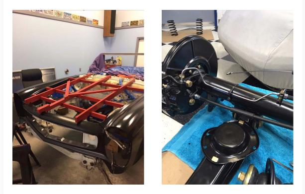
Above left: Since this is a hand-built car, a lot of panel fitting is involved, so a template was made in order to get the hood opening correct. Above right". Stainless brake lines were made to replace the original steel lines.
