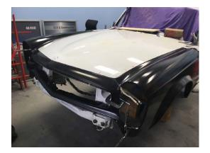
Above left: All parts were bead-blasted, painted, and reassembled with new bushings, etc. Above right: Fitting the hood for testing before final welding.
