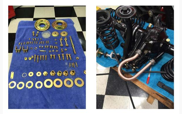
Shown above on left: Many of the parts were sent out for electroplating. Above on right: The cooling pipe for the rear differential had to be re-routed to fit the W113.
